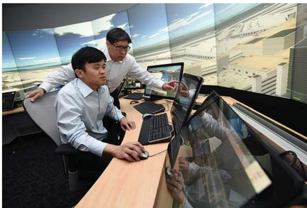
Figure 1. In the Smart Digital Tower Concept, Video Feeds Projected onto an Array of Connected Video Screens Mimic the Controller’s Out-the-Window View from an Air Traffic Control Tower
